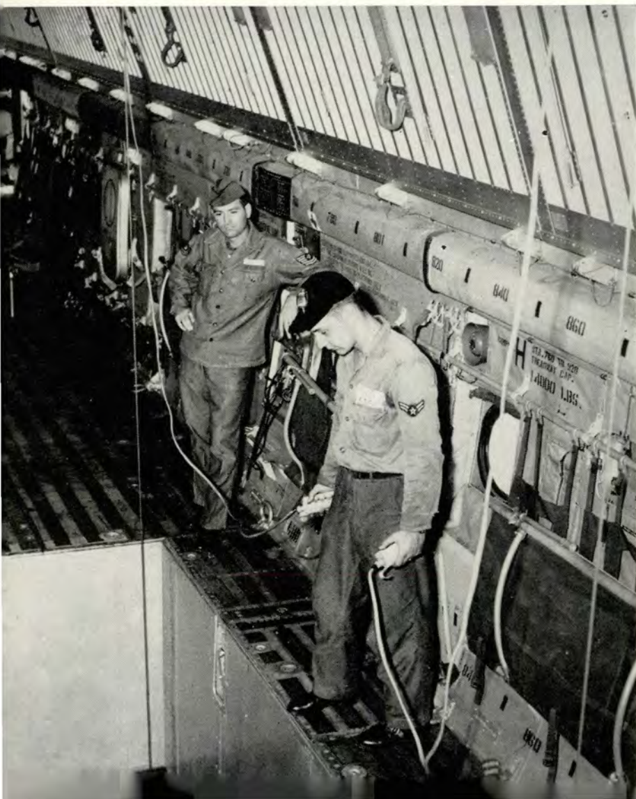
Above, after landing a visual inspection is performed as part of the post-flight procedures. Below, even the Loadmaster is checked for compliance with SOPs.
