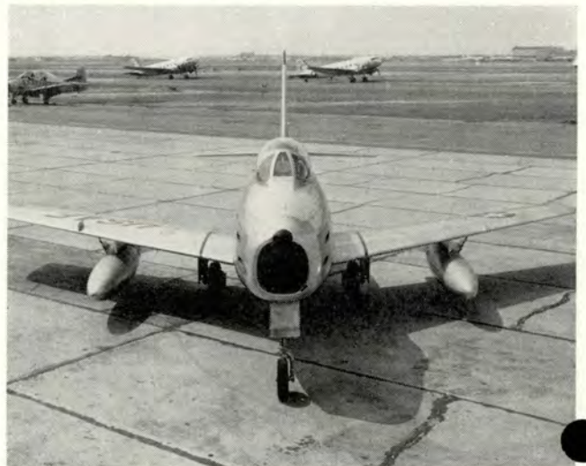
The F-86H is shown with the hard, extended leading edge wing and with the extended slatted wing.
