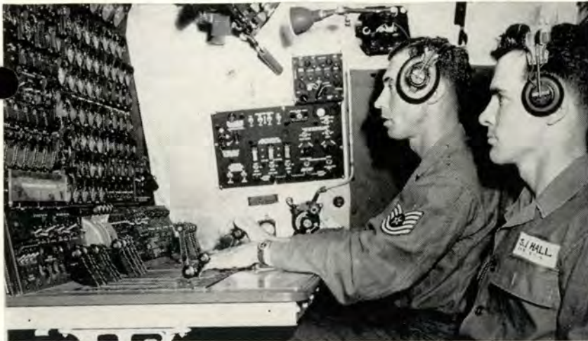
Engine analysis procedures are performed by the Flight Engineer as a stand-board member looks on. Discrepancies in techniques are discussed later during post-flight critique.
